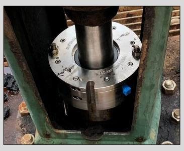
**After:** Split Air Mizer shaft seal installed using existing packing follower bolts
