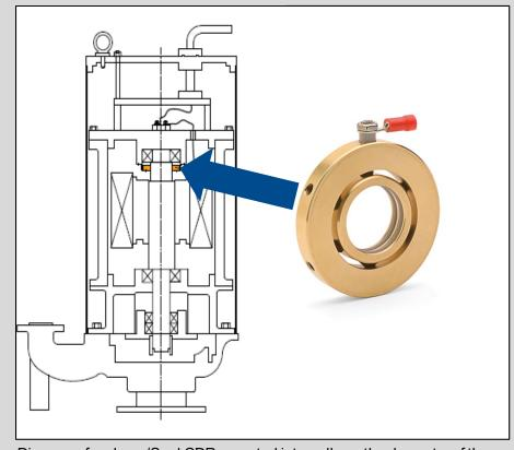
Diagram of an Inpro/Seal CDR mounted internally on the dry motor of the submersible pump
