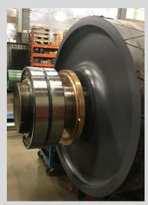
Inpro/Seal Pillow Block Bearing Isolator Installation
