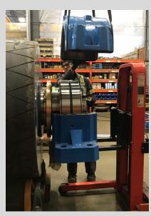
Inpro/Seal Pillow Block Bearing Isolator Installation
