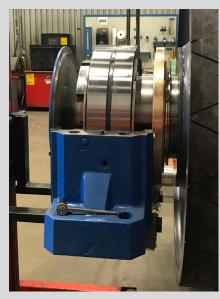
Inpro/Seal Pillow Block Bearing Isolator Installation
