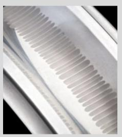
Electrical Discharge Machining (EDM) on the bearing race
