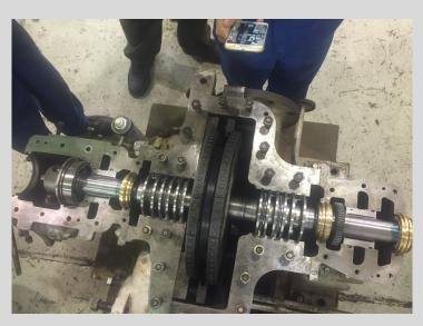
**After:** Installation of Sentinel Floating Brush Seals and Bearing Isolators
