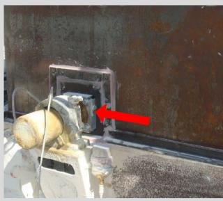
After: Inpro/Seal Air Mizer CEMA shaft seal installed
